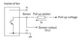
$V_{CE} = +27.6 \text{ V max}.$  $Ic = 5 \text{ mA max.} [V_{OL} = V_{CE} (SAT) = 1.0 \text{ V max.}]$
