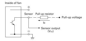
$V_{CE} = +27.6 \text{ V max}.$  $Ic = 5 \text{ mA max.} [V_{OL} = V_{CE} (SAT) = 1.0 \text{ V max.}]$
