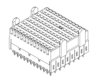
II. THE HOUSING WILL WITHSTAND EXPOSURE TO 260°C PEAK TEMPERATURE FOR 40 SECONDS IN A CONVECTION. INFRA-RED OR VAPOR PHASE REFLOW OVEN
